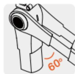
Rotate the tilt-axis of the phone until the intersection angle goes more than 60 degree.
