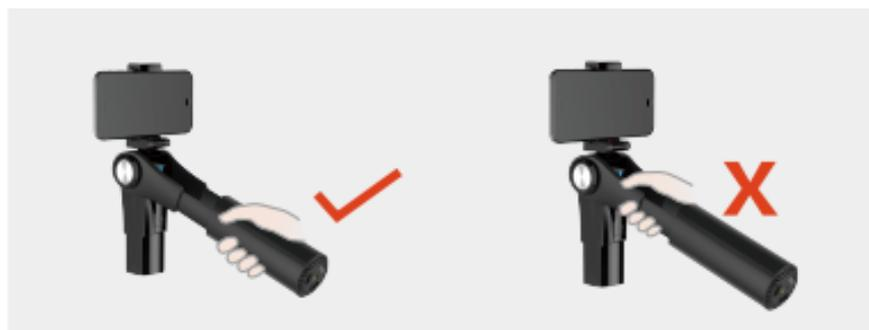
Please hold the handle when using (the picture on the left). When wrongly hold on the middle part (picture on the right), the handle will spin for a while and stop, and trigger the standby mode, all the motors stop working.
