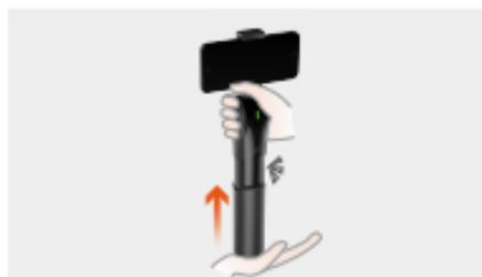
When you want to collapse the gimbal, grab the top part with one hand and align the handle, then use your other hand to tap push the bottom of the handle. Don't put your hands near the middle to avoid getting pinched.
