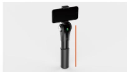
Collapse the tilt-axis to the grip, the gimbal will enter standby mode, and all the motors will stop working.
