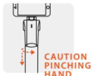
Twist 90° and then pull out (be careful of pinching hand when collapse the handle).
